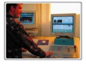
The most realistic "hand on" operating experience comes from instegrating the simulator software into a press console.
